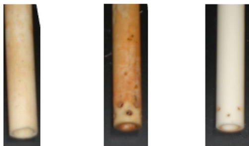
Fig. 4. Tested oxygen gas distributors.
